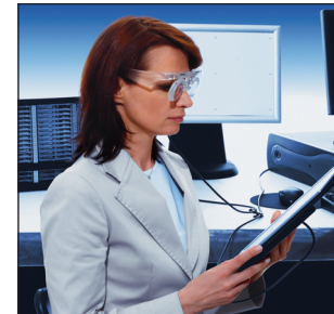
Figure 12. Head-tracking devices are utilized to determine whether a given individual is a “head mover” or an “eye mover” (photo courtesy of Carl Zeiss Vision GmbH).
