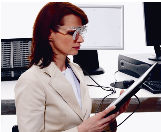
Figure 12. For “biometrically-customized” progressive lens designs, special head-tracking devices are required (photo courtesy of Carl Zeiss Vision GmbH.)
